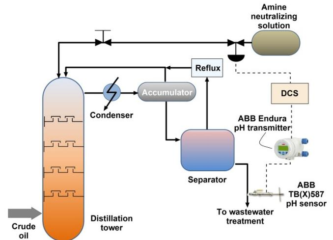
To minimize corrosion, the refinery adds neutralization chemicals, typically organic amines, to the top of the tower. The pH measurement of water coming from the separator serves to control the rate of these additions. The desired pH setpoint is generally between 5.5 to 7. A substantial lag exists between the formation of water vapor within the distillation tower and the pH reading following the separator, making control difficult.
