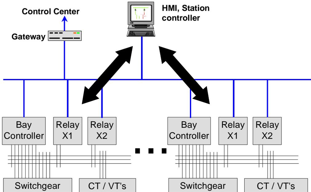
Figure 2 Vertical communication in the substation automation system with hardwired process interface
