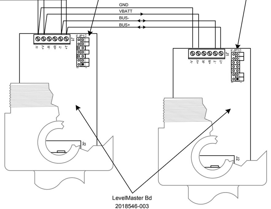
3. The RS-485 buss must be wired in a daisy-chain configuration. Star configurations are not allowed.
