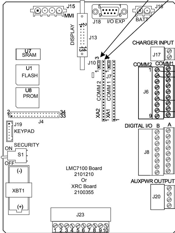
If the LevelMaster board is an intermediate device, and not the last device on the RS-485 buss, set its jumpers to match:
