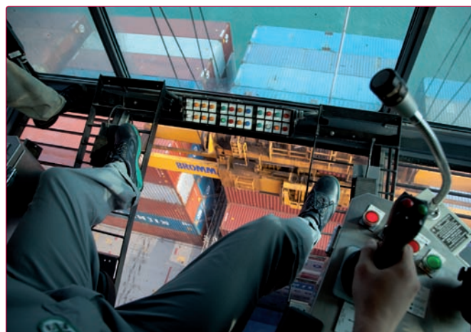
FIGURE 1: No more uncomfortable working positions for crane drivers. The introduction of remote control in STS cranes allows the crane drivers to move to an ergonomic office environment.
