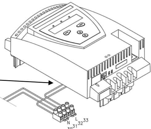
5. On PSTB unit remove the cables from the terminal block.
