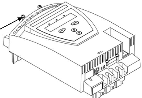
3. Remove the front cover (four screws).
