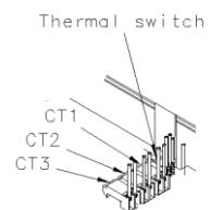
15. Mount the cables from the thyristors and fans on the HV-Board. Be careful how you connect the cables from the thyristors.
