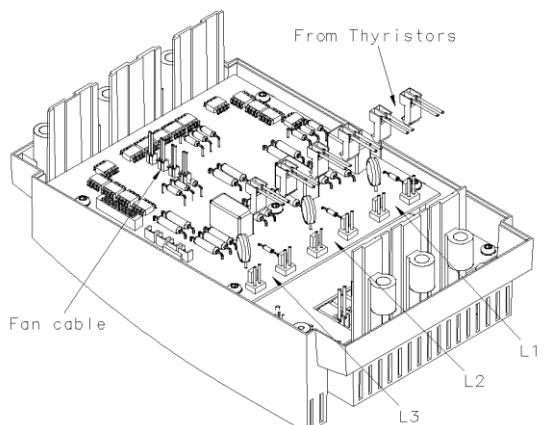
7. If the cables from the current transformers not are marked, mark them with 1, 2 and 3. Disconnect the cables on the LV-Board from the thermal switch and current transformers.
