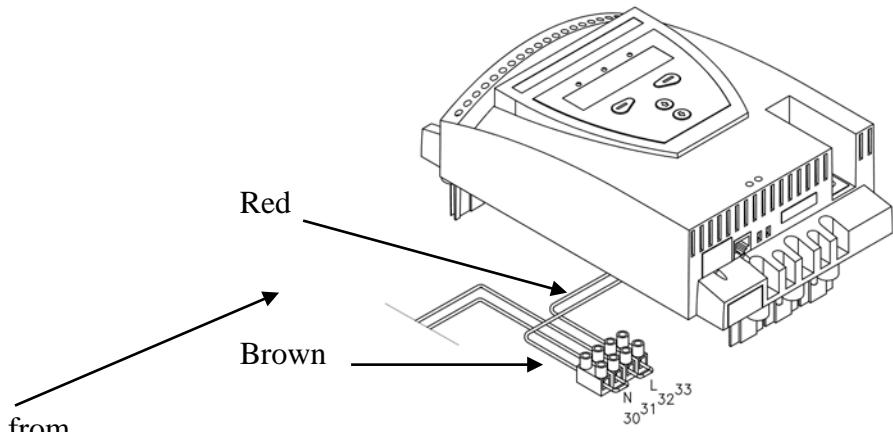
13. On PSTB units, reconnect the cables from the terminal block. **Be careful how you connect the Red (L) and Brown (N) cable.**
