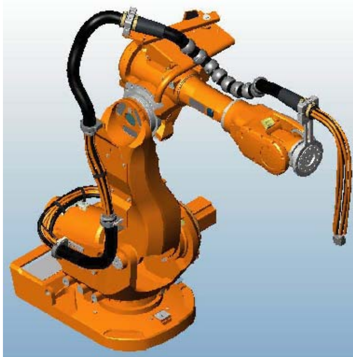
Figure 66 DressPack Upper/Lower arm Spot Welding (option 778-2 and option 781-1).
