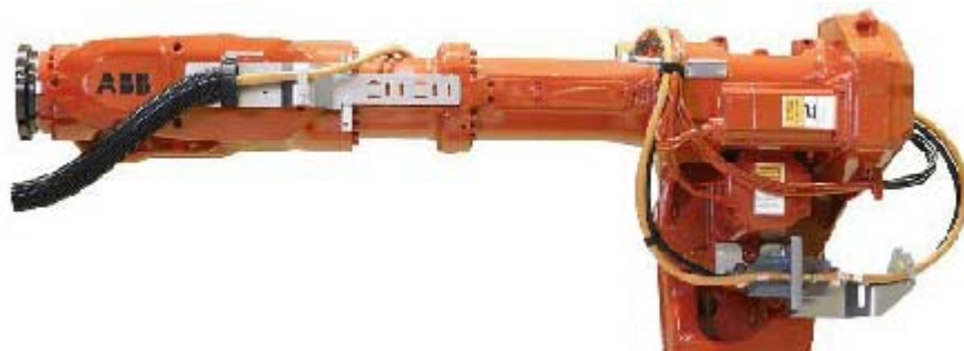
Figure 64 DressPack Upper arm. Axis 3 to 6, Material Handling (option 778-1, option 780-3 and option 798-1).
