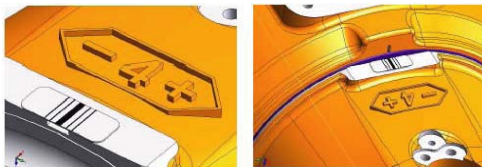
Figure 123 Position for synchronize lables, Axis 4.
