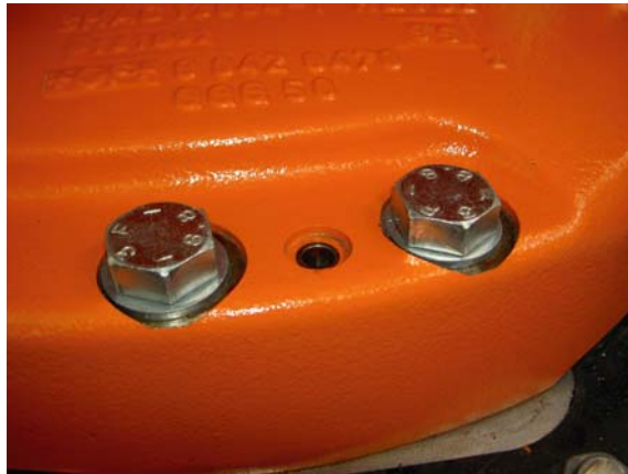
Figure 13 Four Ø12 H8 (depth 12) on radius 400 mm from axis 1 center on robot base.
