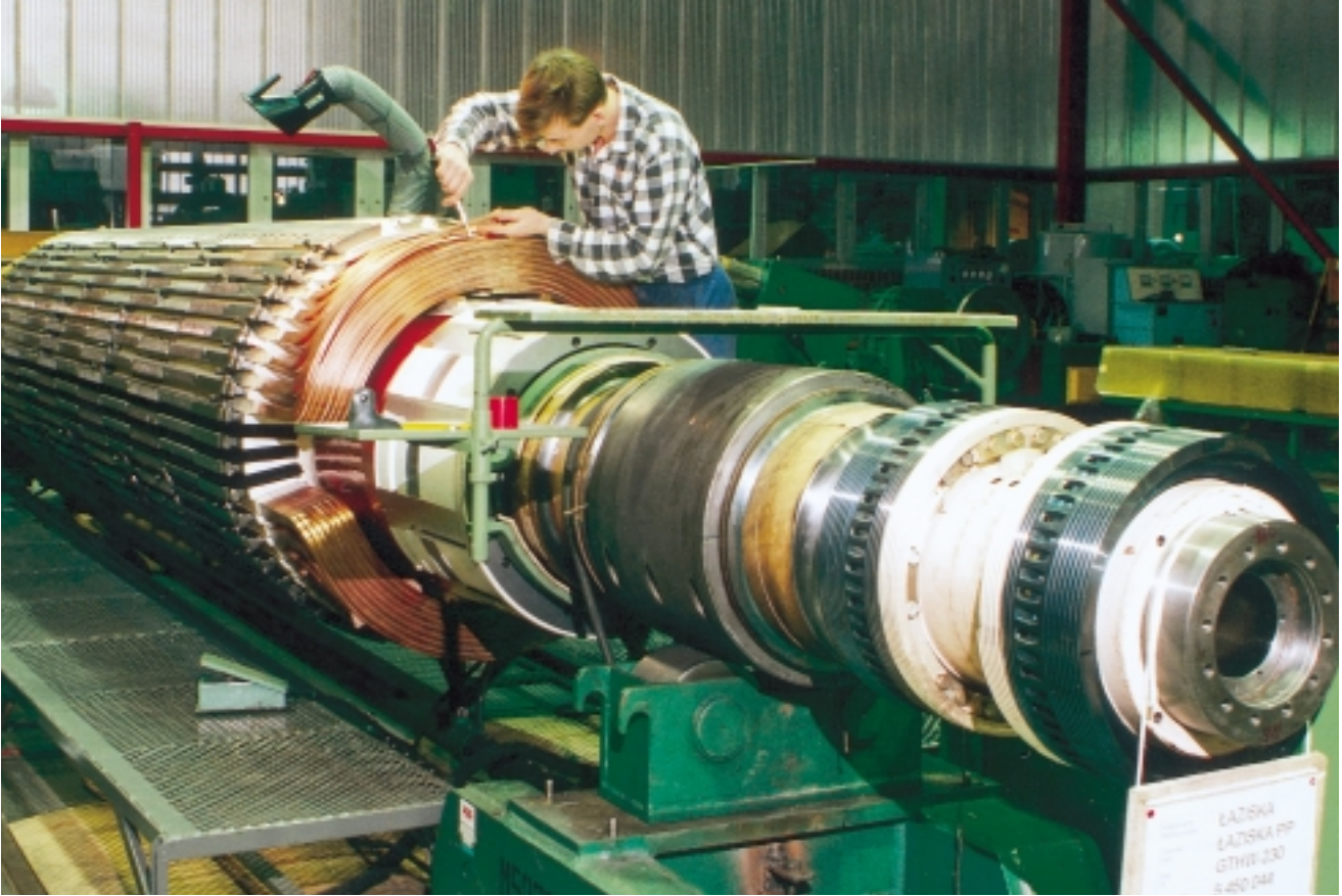
Retrofit work being carried out on a rotor for Laziska power plant (Poland) in the factory of ABB Dolmel, Wroclaw
