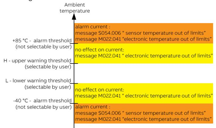
**Warning.** Message M022.041 appears when one of FE or CB temperature exceeds the limit L or H. Alarm message S054.006 appears when one of FE or CB temperature exceeds the limit of -40°C or +85° (different values could be set only in factory on request). For additional details and settings see Add01.
