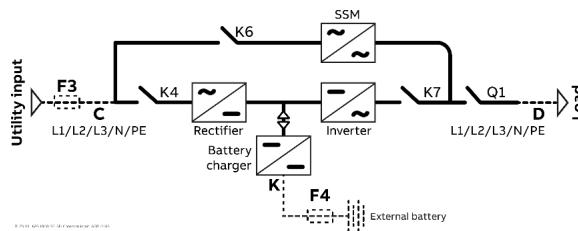
Dual Input Utility Configuration Rectifier &amp; Bypass
