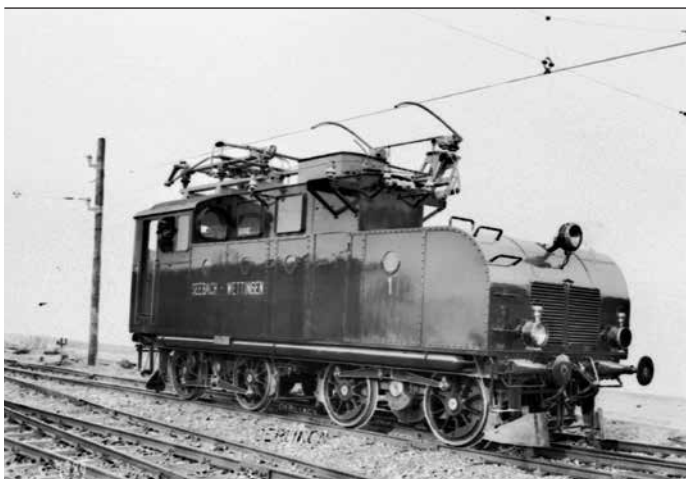
3 MFO experimental locomotive no. 1 with rotary converter and DC traction motors
