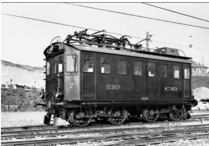
4 MFO experimental locomotive no. 2 with single-phase traction motors
