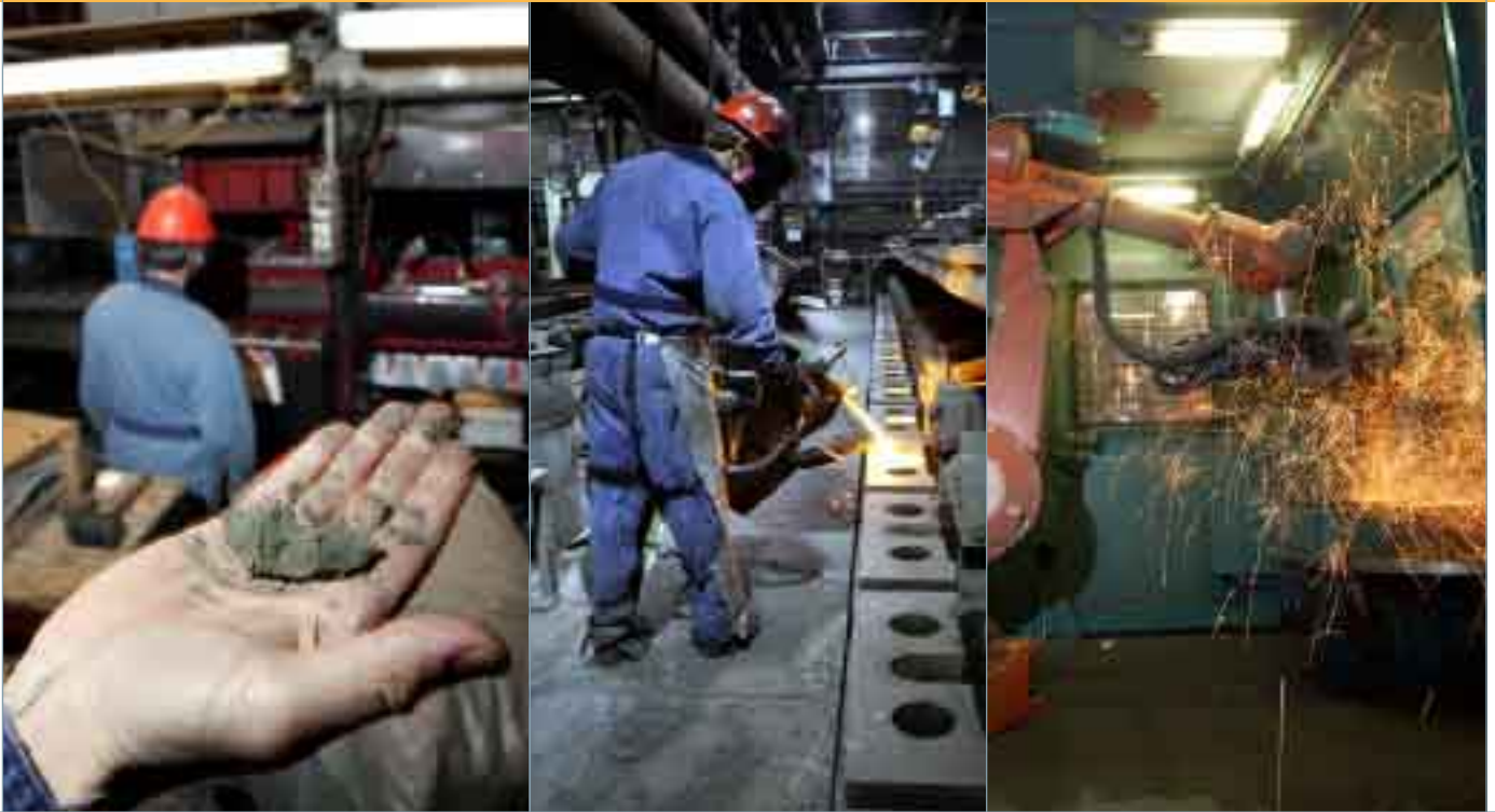
Iron casting at Lethbridge is made easier with the help of robots, who have taken over the heavy job of grinding, right. At left, the sand used in the casting.
