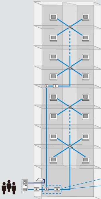
System controller + gateway (auxiliary power supply mode)
