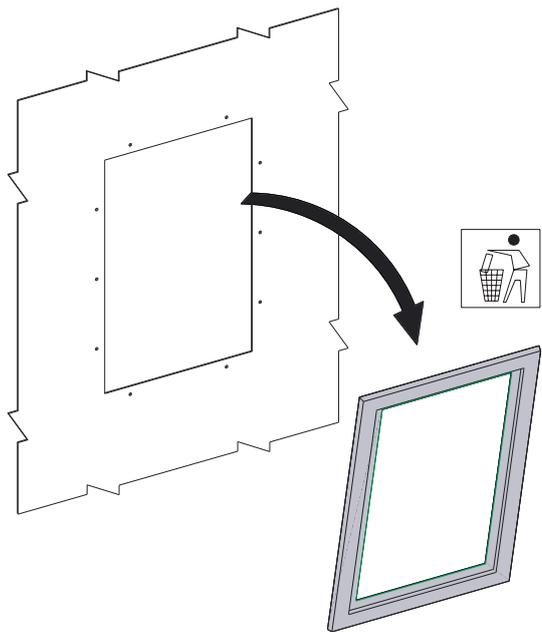
**31** Position the adhesive template on the door and make sure that desired edges perfectly matches the respective existing door cutout edges.
