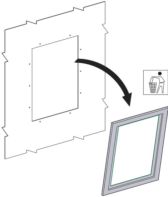
**29** Position the adhesive template on the door and make sure that desired edges perfectly matches the respective existing door cutout edges.
