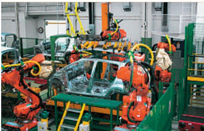
**5** Even car body framing operations are done by ABB heavy load robots in the FlexFramer.
