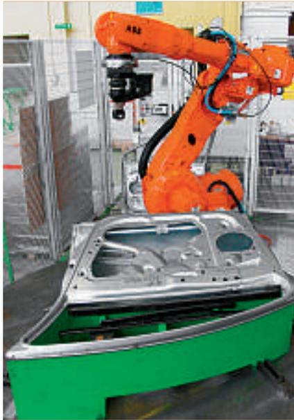
A large part of the body shop, including underbody, framing line and respot was installed in 2003. In addition, front end, central and rear floor assembly lines were also provided. Over 100 FlexiCells are used in the production units and because they were fully tested by ABB prior to shipping and then shipped whole to the plant in Spain, the total installation and commissioning time needed for the cells was minimized.
