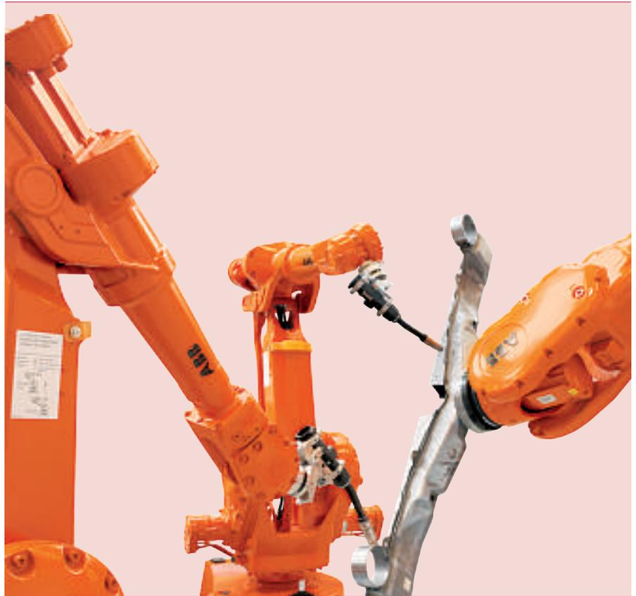
dinate systems of each of the coordinating devices as relative to the work-object held in the handling device. When the work-object moves, the other devices move in symphony.
