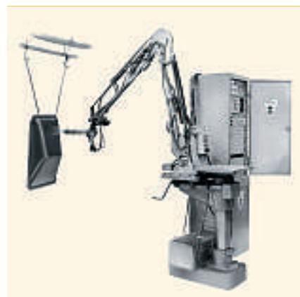
“pendulum” configuration with the arm suspended from a pivot. The arm’s moving masses were concentrated at the pivot, minimising the moments of inertia and resulting in accelerations of 2g within a working envelope much larger than possible with a SCARA.
