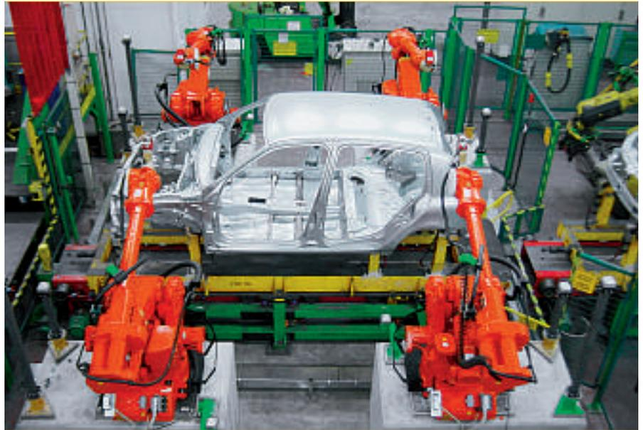
2 Accuracy and repeatability: the work of most industrial robots is repeatable but not accurate. RBMS provides them with the means to hit the centre of the target every time.
