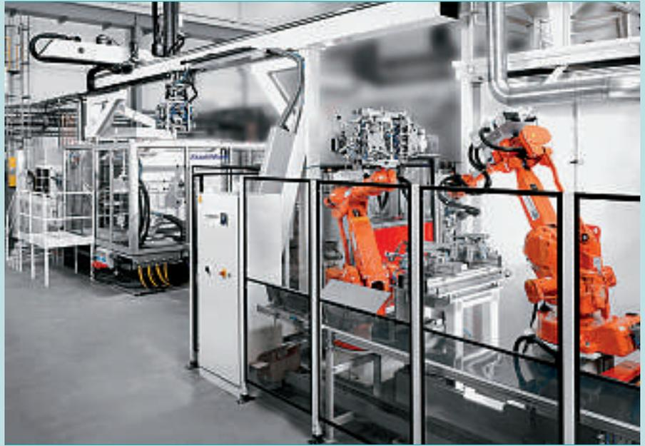
Axes 4 and 5 can rotate through 360 degrees. As a result, the components do not have to be rotated or put down during the cutting process
