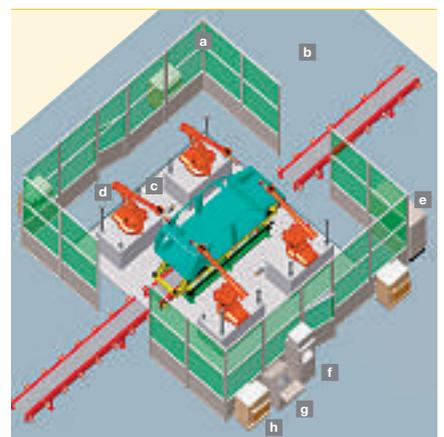
The base plate is a concrete slab. This provides a metrological base and is protected against vibrations from the workshop floor by a peripheral joint. It is not connected to the enclosure for the same reason. The base plate is, however, linked to the robot risers (also concrete) to provide common rigidity. Calibration monuments are attached to the risers assuring stability of geometric relations over time. The monuments themselves are made of silicon carbide for low thermal expansion.
