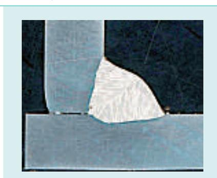
shows that the simulated weld profile is extremely close to its real weld counterpart **2**.
