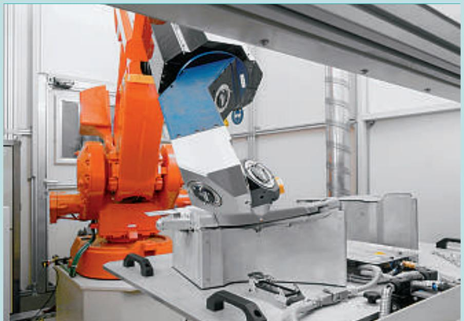
The turntable moves the components into the cell, where they are cut by a Robocut A 300 laser robot developed by Robot-Technology GmbH. The laser robot is based on an ABB IRB 4400 robot. The CO<sub>2</sub> laser has an inherently stable laser housing with axes 4 and 5, which replace the standard main axes of the robot.
