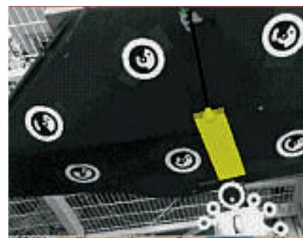
**2** The operator specifies target points using a hand-held device directly in relation to the object to be painted. The simulated result is displayed as a composite image on headworn displays [1].
