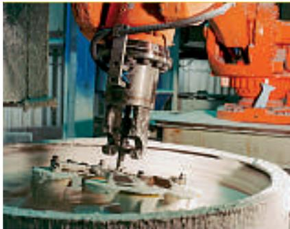
skilled workers to achieve the high casting quality that customers demand. However, there is a definite automation trend. Shell making, where the wax trees are dipped in an alcohol or water based slurry and where the ceramic shells are continuously built using special sand is often robotised 1. Robots are also used for post processing applications, such as grinding and polishing of the cast part.
