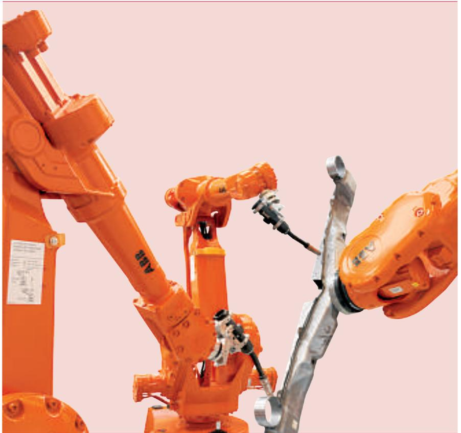
of the coordinating devices as relative to the work-object held in the handling device. When the work-object moves, the other devices move in symphony.
