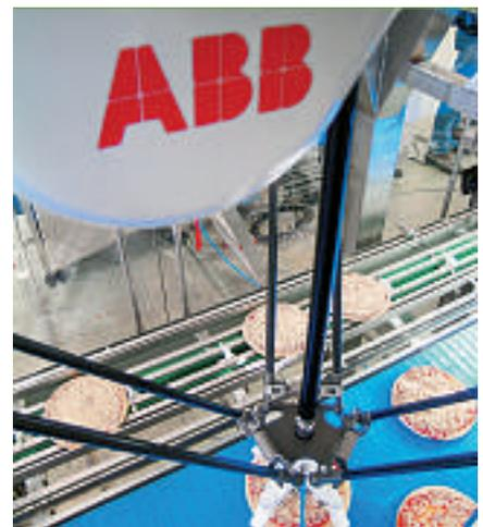
4 The loading system with two FlexPicker robots.
