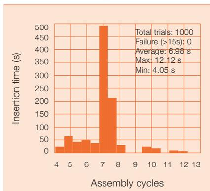
The technology was initially tested on IRB 4400 and IRB 6400 robots, with payloads ranging from 30 to 200kg, used to assemble different automotive powertrain parts. These tasks, which can be considered complex, included inserting forward clutch hubs and the assembly of F/N torque converters **1**. The tests demonstrated consistently superior performance in terms of cycle time, acceptable insertion force, reliability and ease of programming.
