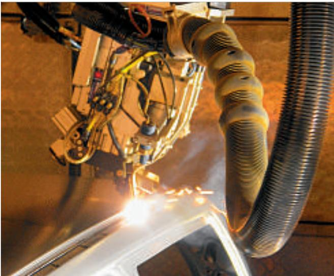
the seam together. Different PD module designs are available depending on the application. For example, a flange joint weld needs a two-wheel configuration – one wheel for every sheet, whereas a single wheel is normally sufficient for an overlap joint.
