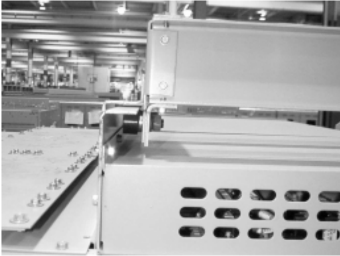
Fig. 4-26. Location of hoist rear rollers
