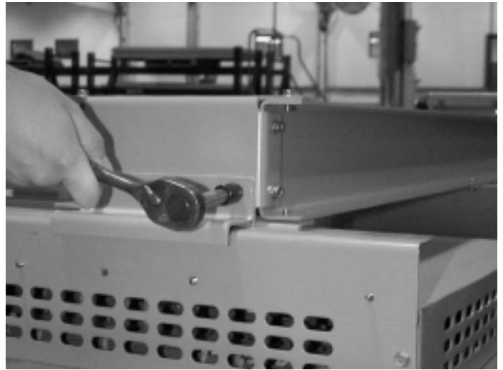
Fig. 4-28. Replacing the runner guide after completion of hoist installation
