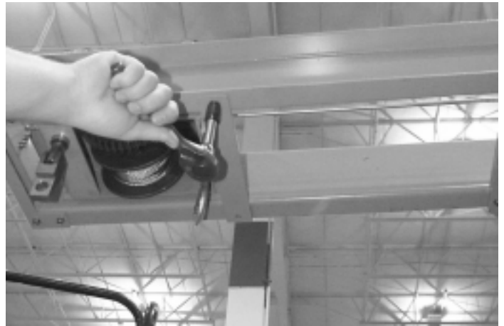
Fig. 4-29. Removing the bracket locking the hoist dolly
