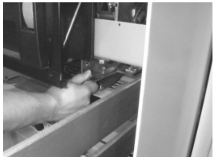
Fig. 5-12. Spring discharge interlock used on manually and electrically operated breakers
