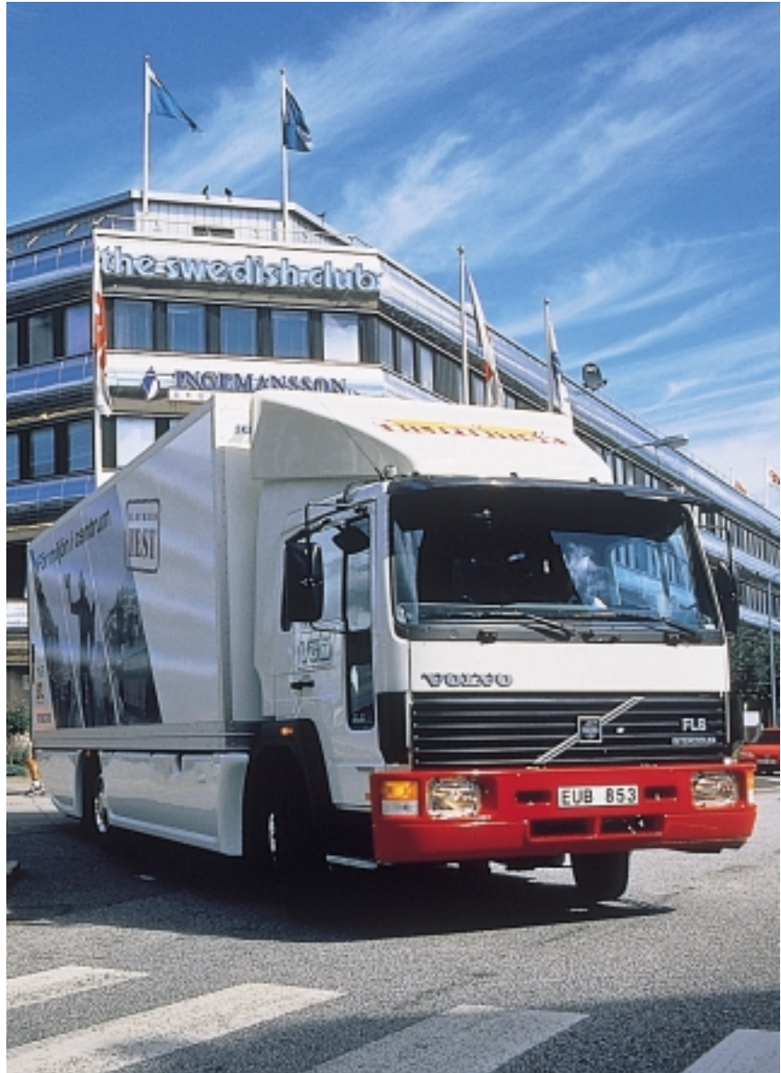
One of the two trucks fitted with a hybrid drive and now taking part in a three-year trial in central Gothenburg, Sweden, where it is being used to distribute goods
