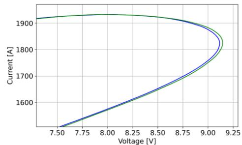
**Fig. 3:** Example of on-state shift, in green the second half sinusoidal current pulse shows an I-V curve with higher on-state voltage compared to the first pulse in blue with the same current conditions.
