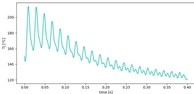
**Fig. 12:** Junction temperature profile obtained from the active short circuit simulation.
