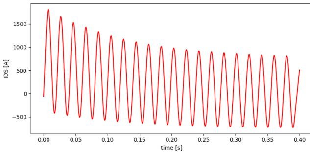
**Fig. 11:** Active short circuit current profile simulated using the PLECS model.
