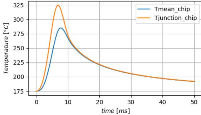
**Fig. 6:** Simulated temperature profiles obtained for the chip body (blue) and junction (orange).
