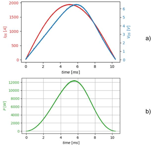
**Fig. 4:** a) Current profile  $I_{DS}$  (in red) and corresponding on-state voltage  $V_{DS}$  (in blue). b) Power dissipated profile (green).
