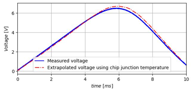
**Fig. 9:** Comparison between measured voltage on a surge current measurement (blue) and the calculated extrapolated voltage (red) by using the junction temperature profile obtained in FEM thermal simulation.
