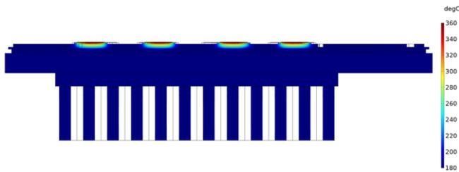
**Fig. 7:** Temperature contour from the thermal simulation of the surge current test at a cross-section of the RoadPak through the HS chips.
