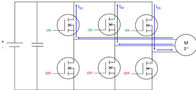
**Fig. 1:** 3-phase PMSM drive with ACS mode with only the high side (HS) of the inverter turned on.
