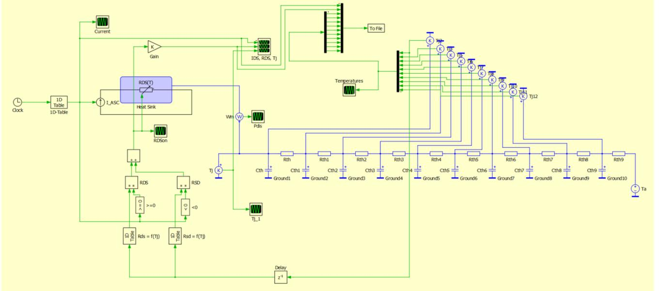
**Fig. 10:** PLECS model for active short circuit or surge current simulations.
