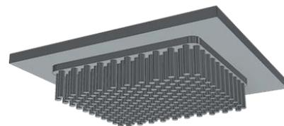
**Fig. 5:** Baseplate and pin fins of a RoadPak module.
