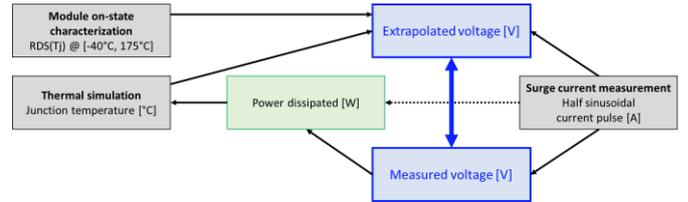
**Fig. 8:** Schematics of the approach followed to validate the extrapolation of the on-state voltage for higher temperatures than the characterized temperatures range.
