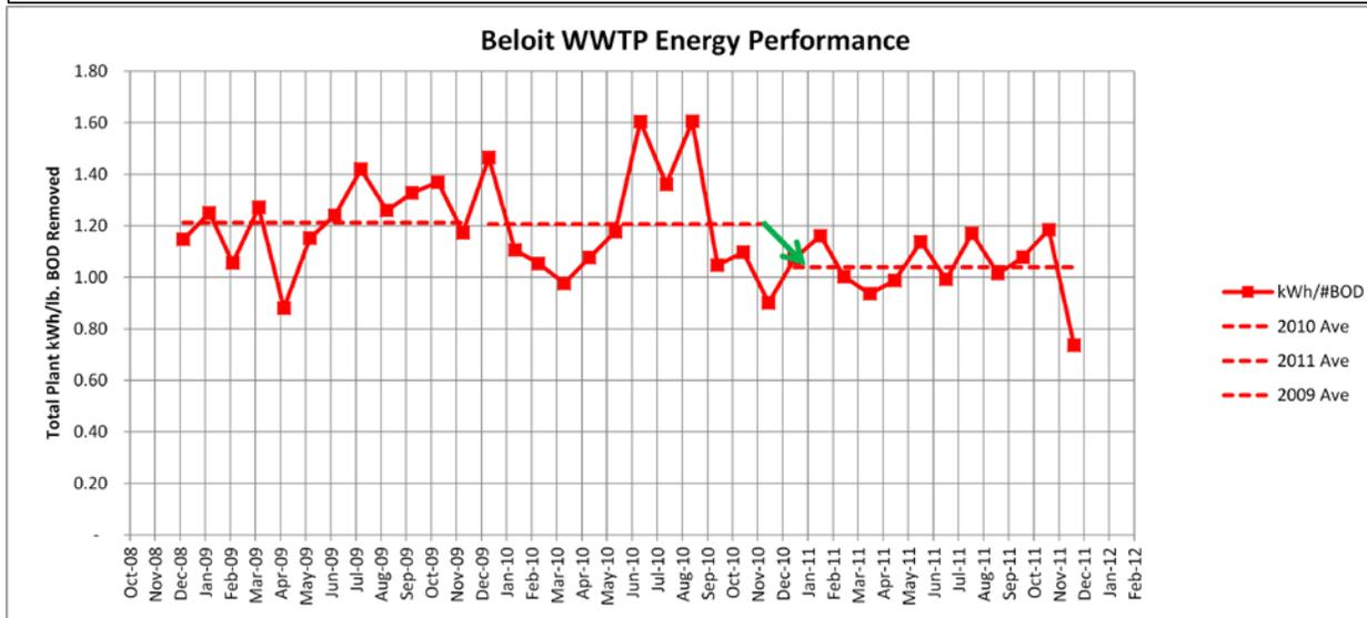
**Conclusions and Recommendations:** The Beloit WWTP shows a successful application of VFDs to aeration blower control. The strategy isn't new, and aeration blowers have been provided with VFD control for some time. (An early installation in Pennsylvania dates to 1989.) However, the introduction of cost effective medium voltage VFDs represents a new class of potential applications for this technology.
