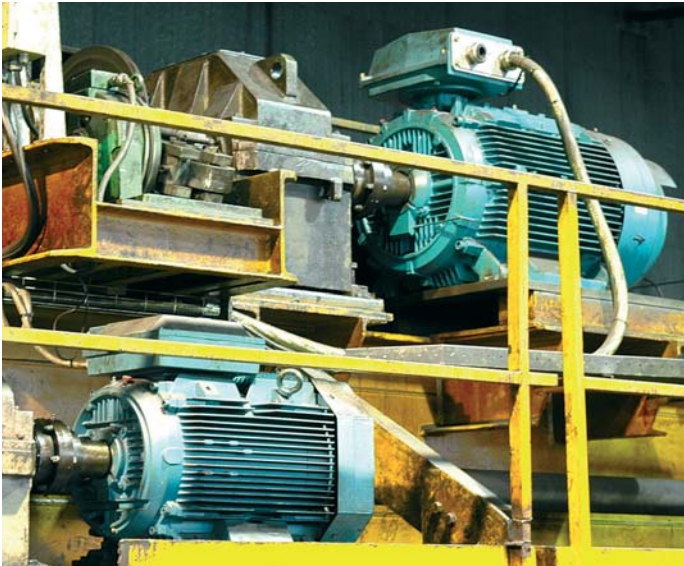
Hoist motors use incremental encoders for accurate position feedback.
