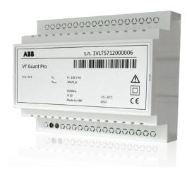
VT Guard Pro is an security device that protects medium voltage inductive voltage transformers against ferroresonant oscillation. Ferroresonance can arise in ungrounded power networks or in the networks where is not directly grounded neutral point. It is designed to be used in open- delta connection of three single-phase voltage transformers. VT Guard Pro (Pro D) fully replace dumping resistor and save space in customer application.
