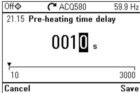
Select Pre-heating time delay between 10 to 3,000 seconds
