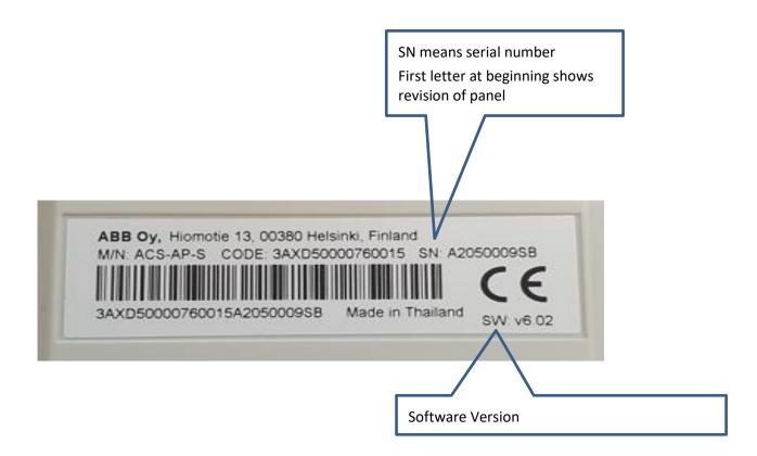
Many of these panels have three different hardware revision groups. See below tables for compatibility. There are two different part numbers with different software depending on the revision of the panel. The software for each revision group is not compatible with other revisions of the panels. For example, Rev K and older software cannot be upgraded to Rev L software Ver 6.xx.
