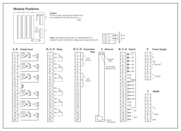
\*Note. 24 V DC instrument power supply must be specified when ordering.
