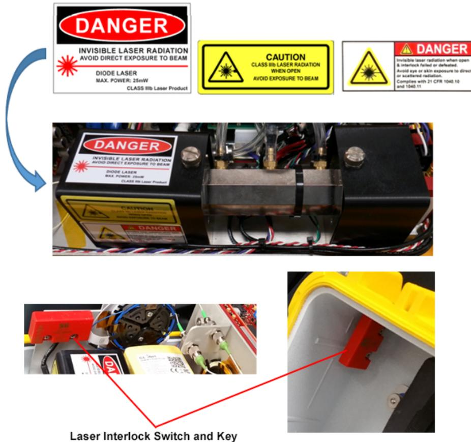
**Figure 2: Laser Radiation Labels and Magnetic Interlock Switch**
