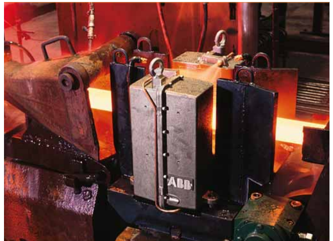
2 U-gauge in operation for dimensional measurement
