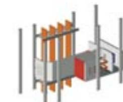
Structural frame of a compartment with moulded-case circuit-breaker in form 4b
