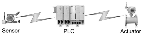
Fig. 5. This picture illustrates a typical scenario of closed loop control, where the sensor provides feedback to the system. Correct functions of all parts (sensor, PLC, actuator, and communication) are required for proper control performance.
