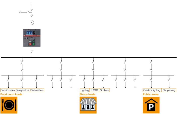
A commercial installation is reported here above: some loads (like HVAC) can be disconnected for a certain amount of time without compromising the plant functions.
