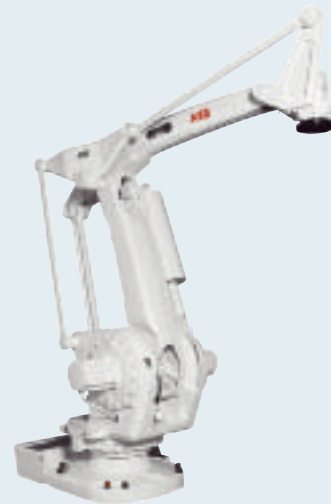
The IRB 660 is designed for palletizing.
