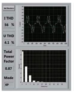
6-pulse drives without any harmonic reduction have a dramatic impact on the power distribution system – in this case the level of input current distortion is 56% and reduces the power factor to .87.
