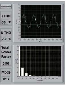
The level of harmonic distortion is reduced when reactors are added to 6-pulse drives, but is still significant. Total power factor is also improved.
