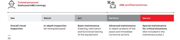
Starting from these levels, we provide a maintenance plan and related activities for circuit breakers, switchgear and relays, where maintenance cycles are diversified for different equipment conditions. For example, for severe conditions we need to reduce maintenance intervals by 50%, while we can increase them by 30% for optimal ones.
