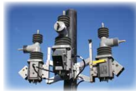
Available in 15-38 kV, the OVR-3SP utilizes three individual single-phase recloser poles for flexible mounting options.
