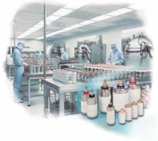
ABB vacuum interrupter clean room
