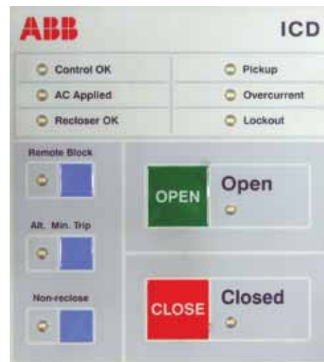
The ICD HMI has large indicator buttons that are easy to read, see and use
