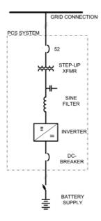
Because of the wide range of battery applications and battery types, ABB will custom design the PCS to fit the specific project requirements. Depending upon the battery type (sodium-sulphur, lithium-titanate, nickel-iron, zinc bromide flow, etc.) the range of DC voltage from fully charged state to fully discharged state can vary widely.
