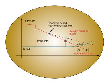
"Insulation material in electrical machines is exposed to thermal, electrical, mechanical and environmental stresses during operation. Over time these stresses cause aging of the insulation material. Aging is represented by the red curve. Stresses from normal operation and abnormal events (such as transients) are represented by the blue curve. When the blue and red curves cross, an insulation failure will occur leading to expensive unplanned downtime."
