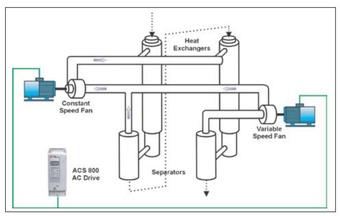
The milk flows in the pipes of the heat exchangers. The hot steam surrounding the pipes makes the water evaporate from the milk. The evaporated water is separated from the milk in the separator. The steam is compressed by the fan and is fed back into the heat exchangers.
