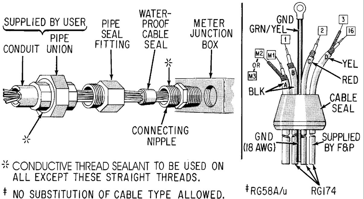
\* CONDUCTIVE THREAD SEALANT TO BE USED ON ALL EXCEPT THESE STRAIGHT THREADS.
