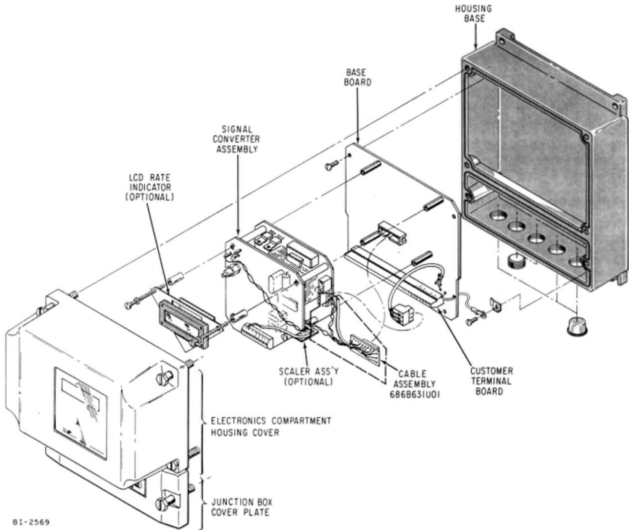
**FIGURE 6-5. EXPLODED VIEW, REMOTE MOUNTED SIGNAL CONVERTER**
