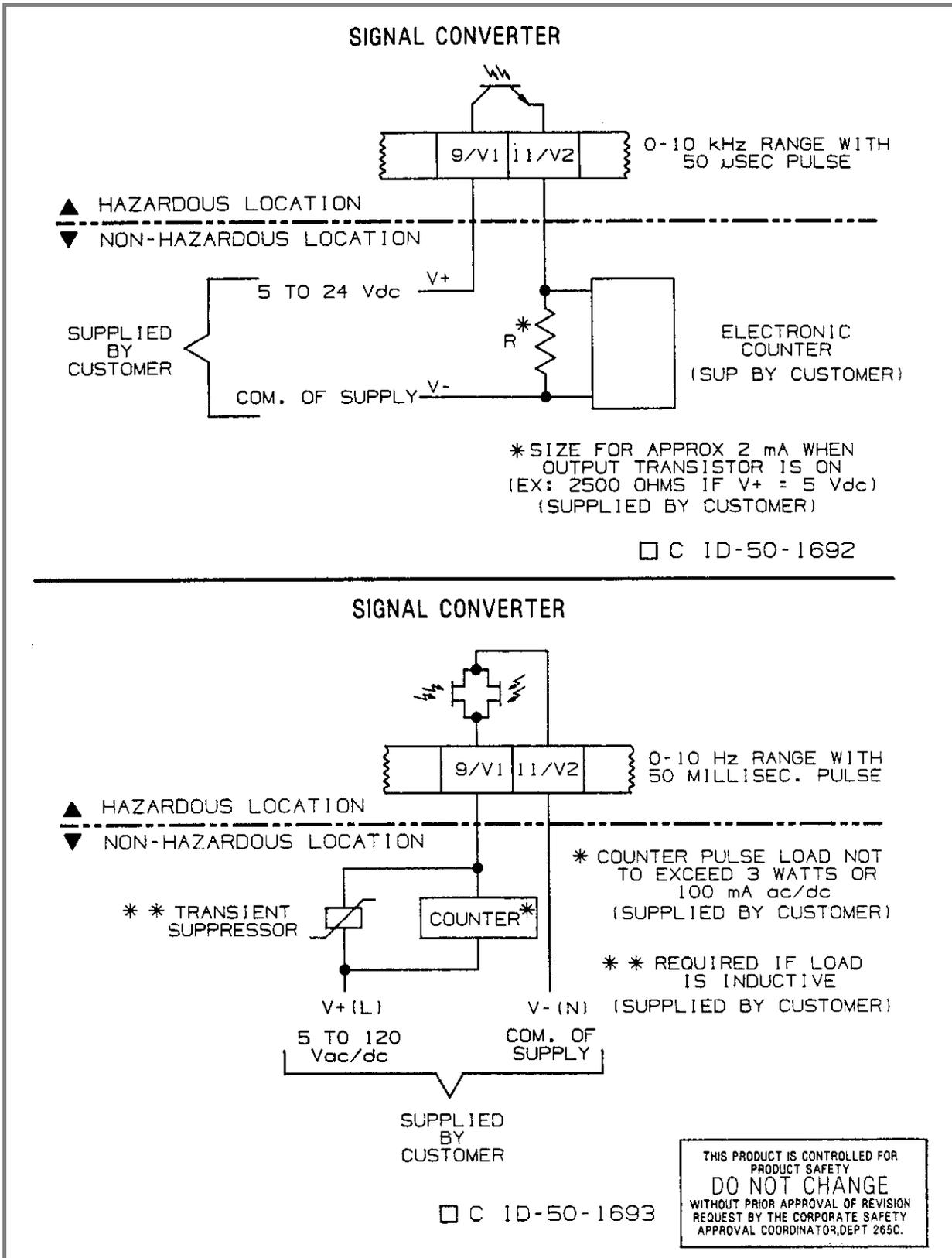
**FIGURE 2-10. INTERCONNECTION WIRING DIAGRAM;
