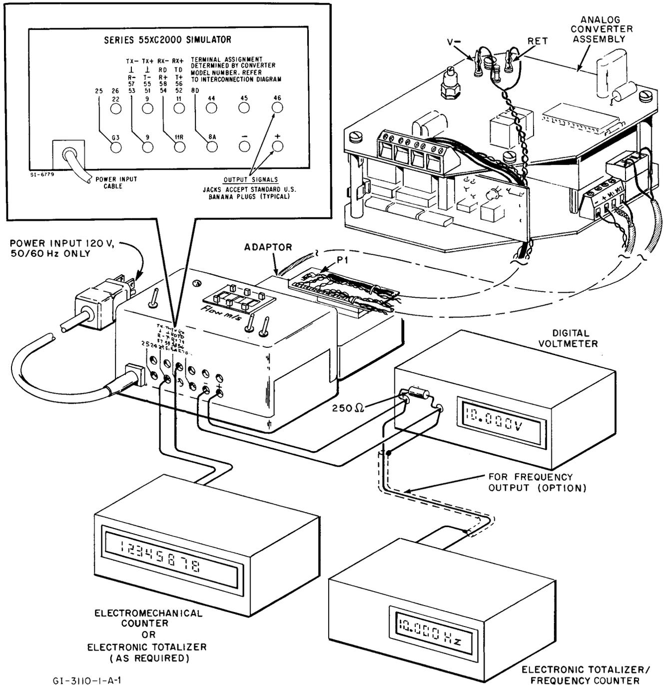
FIGURE 4-2. TEST WIRING USING THE 55XC2000 SIMULATOR
