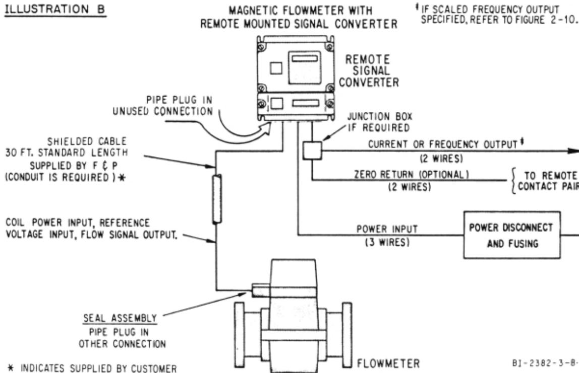
**FIGURE 2-2. ELEMENTARY INTERCONNECTION DIAGRAM**
