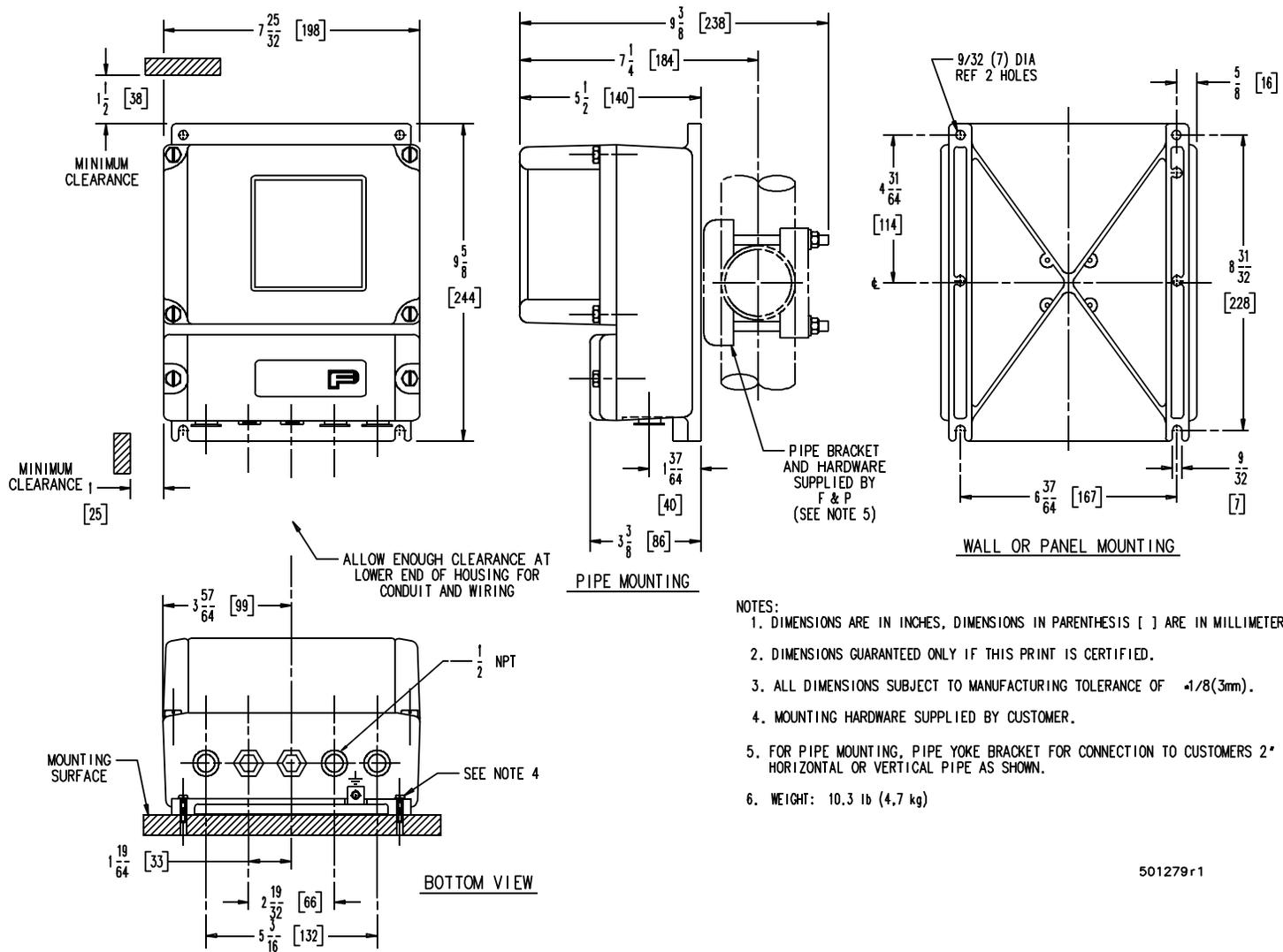
FIGURE 2-1. OUTLINE DIMENSIONS, REMOTE MOUNTED SIGNAL CONVERTER
