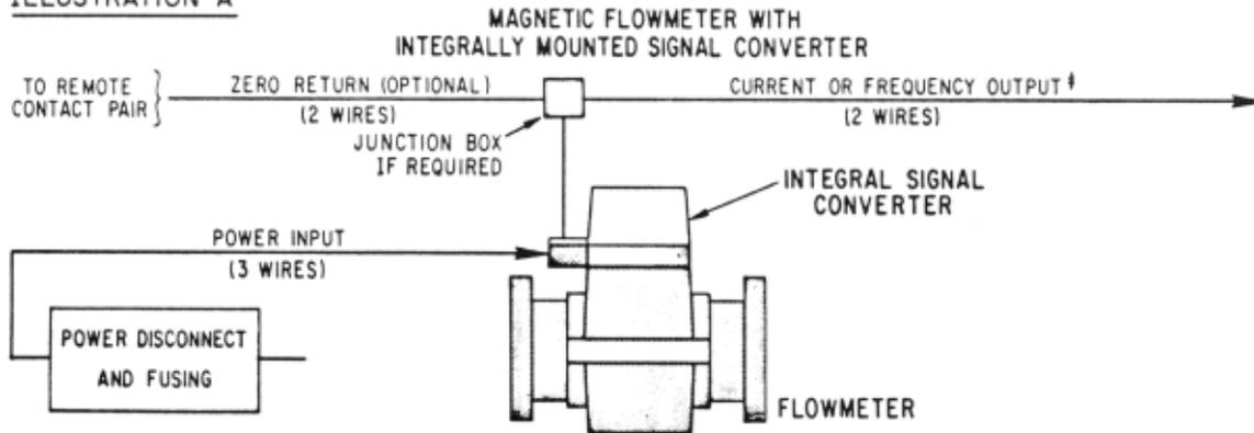
NOTE: EXCEPT WHERE SPECIFICALLY STATED; POWER, OUTPUT AND ZERO RETURN CAN BE RUN IN COMMON CONDUIT.
