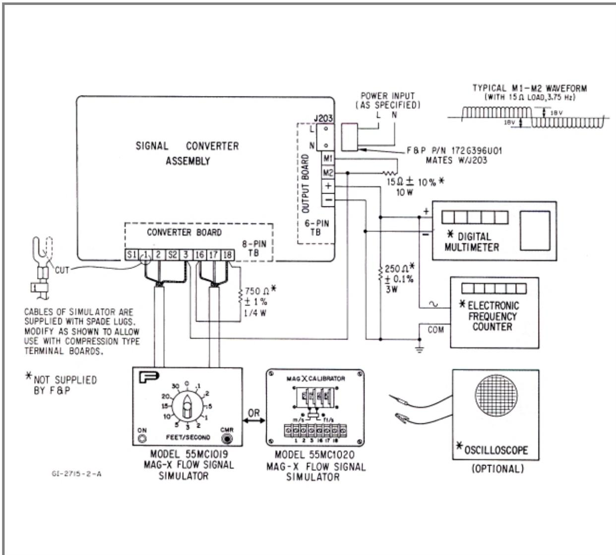
FIGURE 4-1. TEST WIRING USING THE 55MC1019/1020 SIMULATORS
