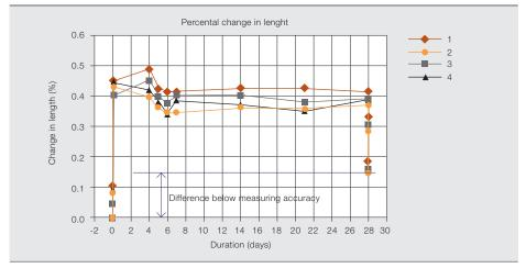
These were performed with the embedded pole type PT1 at 5000 N and 85 °C, and show that no measurable deformation occurred. The jump at the beginning and end of the test period reflect heating from room temperature and the return to it.
