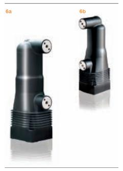
As the PT1 is used in medium-voltage systems, the general requirements are laid out in IEC 62271-100. These are all fulfilled or exceeded by the PT1. The pole fulfills the highest qualifications known by the standard, namely M2 (mechanical endurance), E2 (electrical endurance) and C2 (capacitive switching for back-to-back and cable switching operations).
