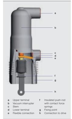
circuit breaker must fulfill three functional criteria: It has to handle nominal current, break short-circuit current, and block voltages exceeding the rated voltage level.
