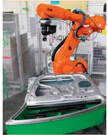
1 Spot-welding robot in car manufacturing
