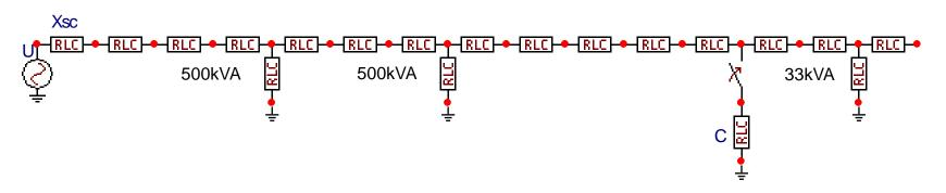
One capacitor switchable located about 80% down the line varying from 200 kvar to 800 kvar
