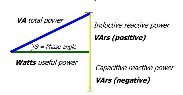
$VA = Volt Amperes = SQRT (Watts^2 + VArs^2)$ For  $\Theta = 45^{\circ}$ , If W = 1 then VAr = 1VA = SQRT(1+1) = 1.4 VA
