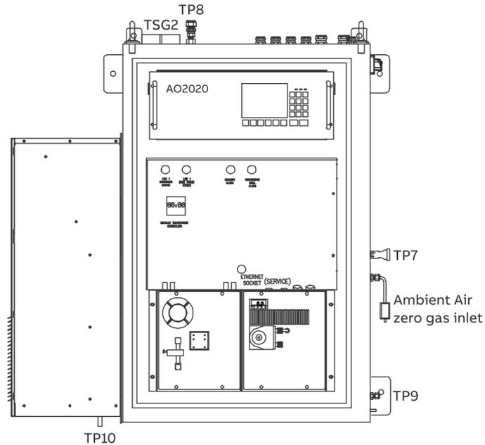
Figure 23: Gas connections GAA610-M
