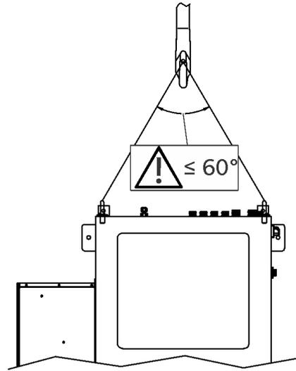
Figure 6: Lift-Up the analyzer cabinet
