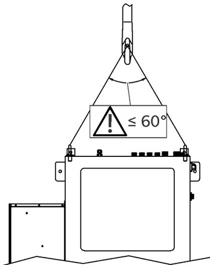
Figure 22: Lift-Up the analyzer cabinet
