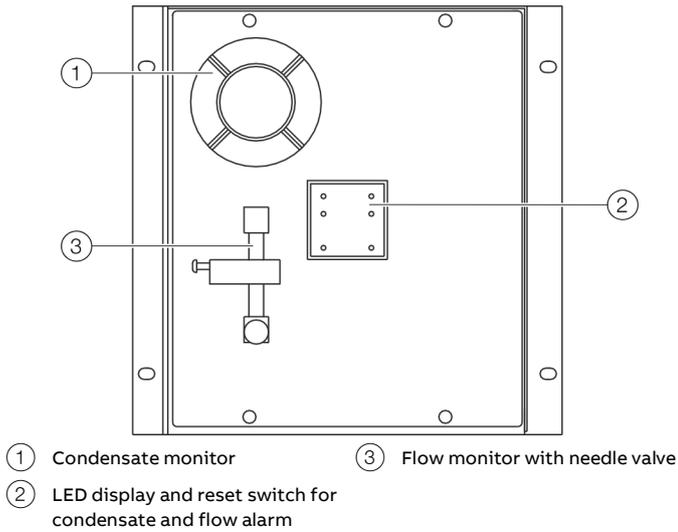
Figure 4: Sample Gas Feed Unit SCC-F
