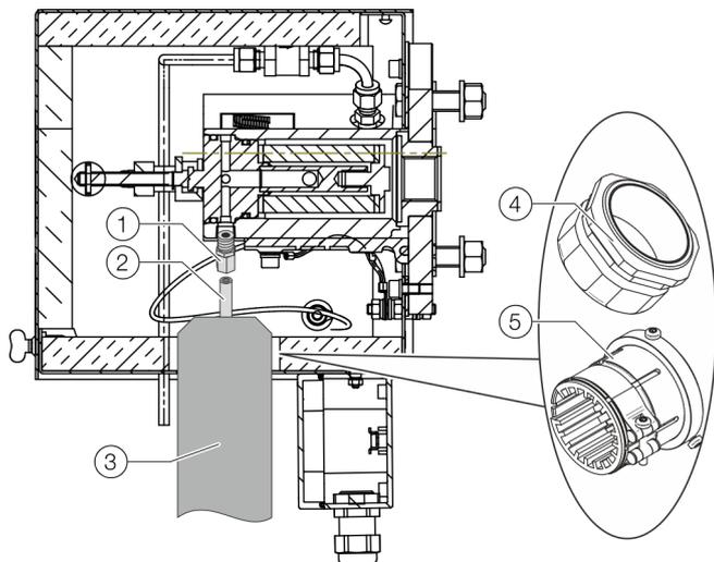
Figure 13: Connection of the heated sample gas line
