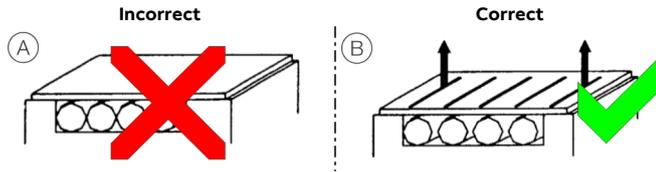
Figure 15: Laying in ducts or shafts
