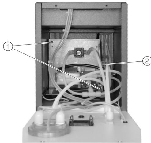
4. Take off the pump hoses and clean the outside of the pump.
