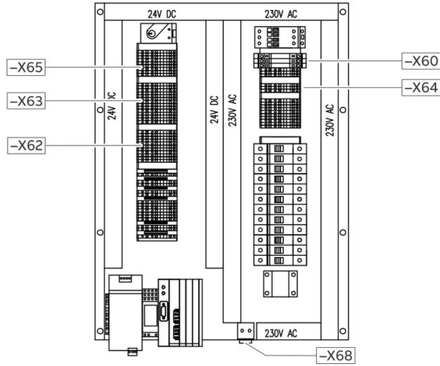
Figure 26: Location of the terminal strips on the back plate of the analyzer cabinet
