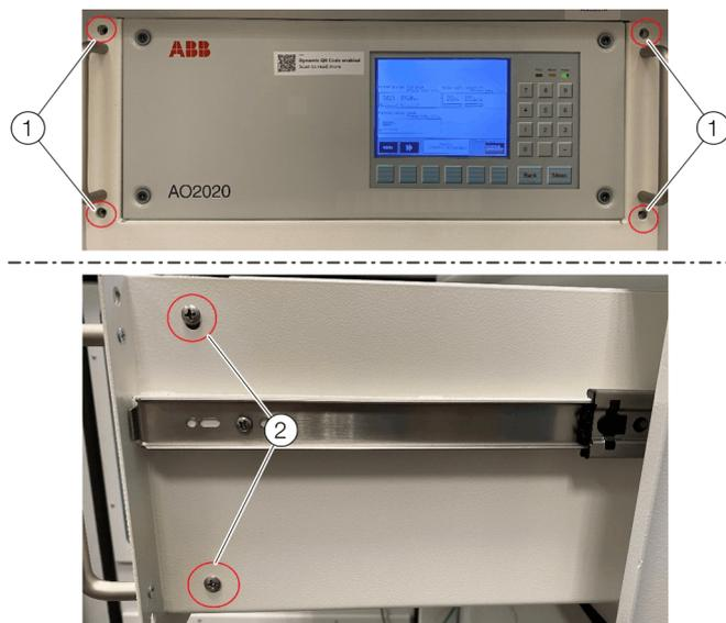
Figure 60: Front AO2020, mounting AO2020 on housing (right)
