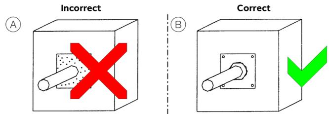
Figure 18: Wall break-through
