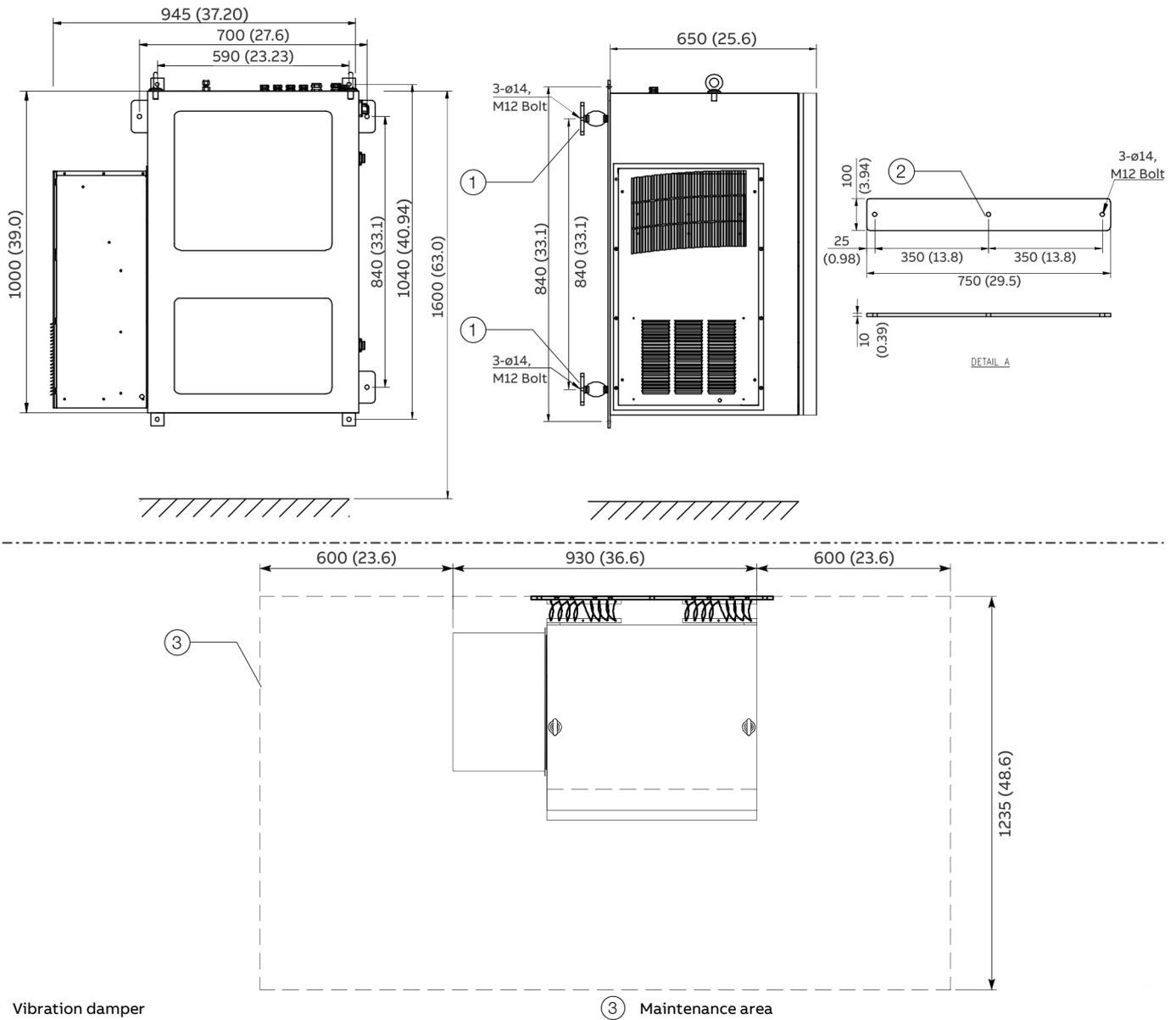
Figure 8: Dimensions analyzer cabinet, mm (in)
