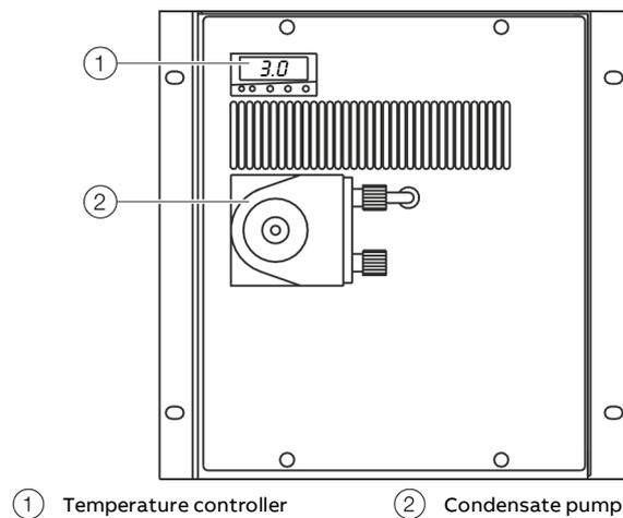
Figure 3: Sample Gas Cooler SCC-C
