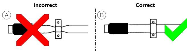
Figure 20: Mounting brackets
