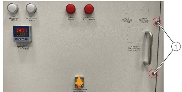
Figure 53: SCC-C cover screws
