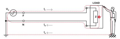
Insulation fault and current path
