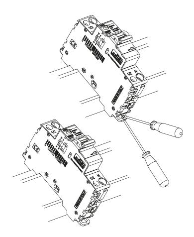
Using a screwdriver, pull down the DIN rail clip at the bottom, tilt the device, and place the rear upper recess on the top part of the rail, move the bottom part of the DS301C towards the rail, remove the screwdriver from the clip – the device is now installed.
