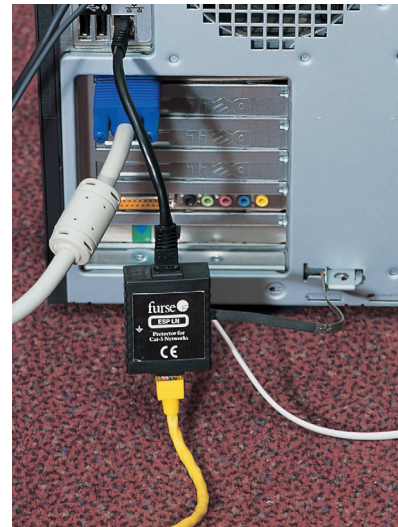
Figure 2: ESP LN installed on the network connection to a PC. Note the black earth lead connection to the chassis of the PC.
