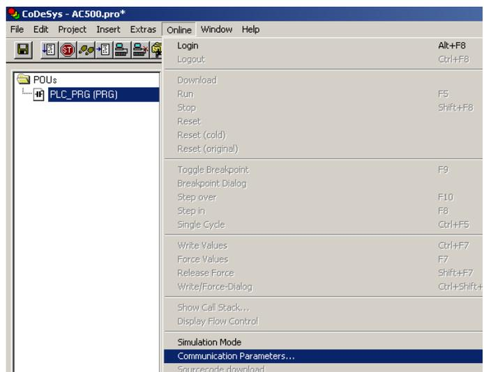
15.2 In the **Communication Parameter** dialog box, click **New...** button to add a new channel. Type the name for this channel. In this example below, **192.168.3.35** is the name for this channel.
