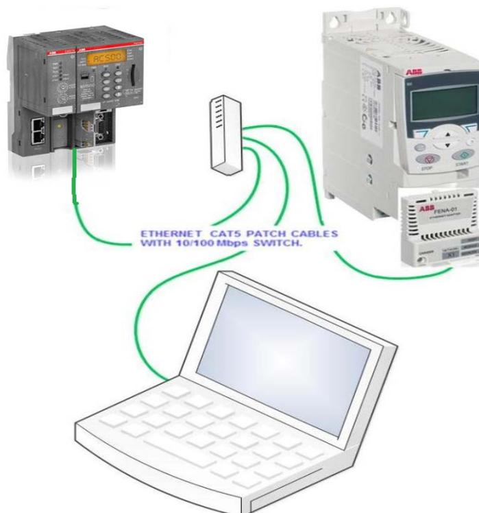
1. Install the FENA-01 field bus module into this ACS355 drive
