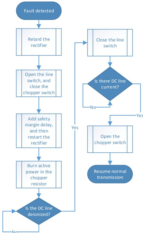
Figure 9, flowchart for DC Chopper operation
