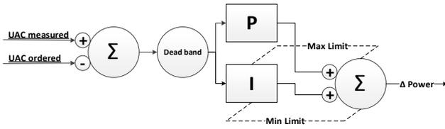
Figure 4, AC voltage amplitude controller
