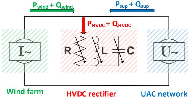
Figure 2, simplified onshore wind power transmission
