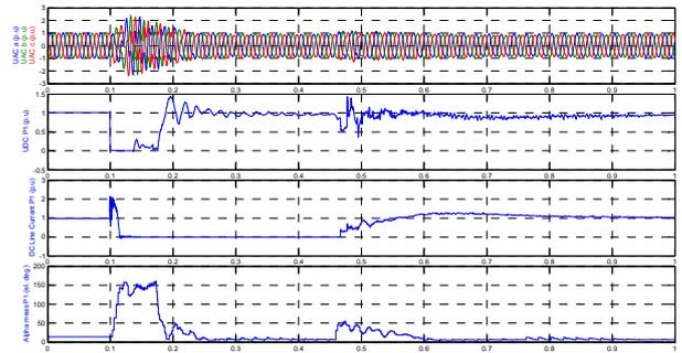
Figure 10, DC fault in pole 1, while pole 2 transmits power
