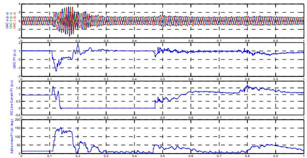
Figure 11, low impedance three phase AC fault at the inverter
