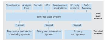
The figure shows information and alarm management tools utilizing a data store integrating technial systems and computerized maintenance management systems to offer unparalelled decision support.
