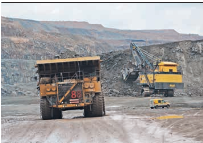
3 Massive, 100 ton trucks with wheels 3.4 m high are used to carry 200 ton loads to the crusher inside the pit at Aitik. Photo by Peter Tubaas.
