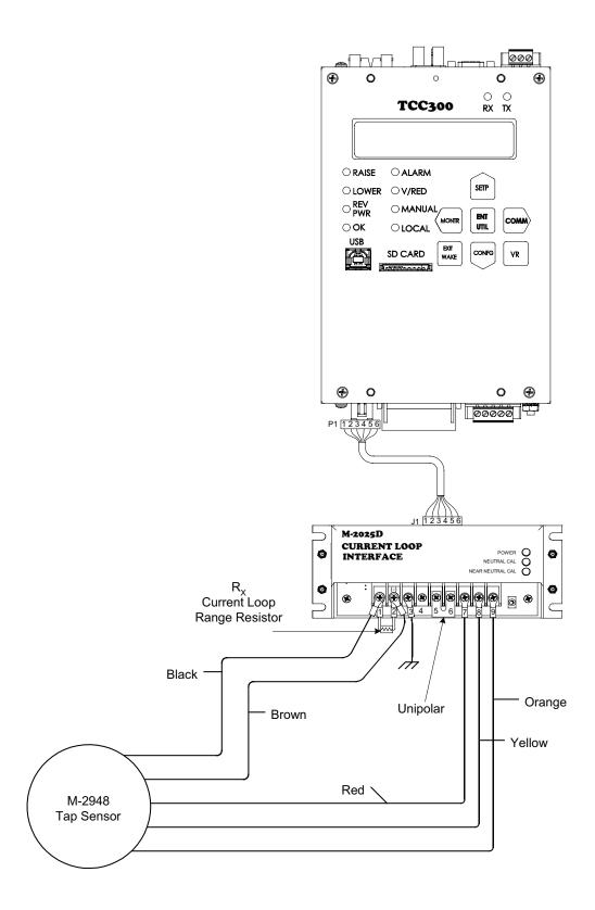
Figure 5 Typical M-2025B(D) External Tap Position Interface with M-2948 Tap Position Sensor
