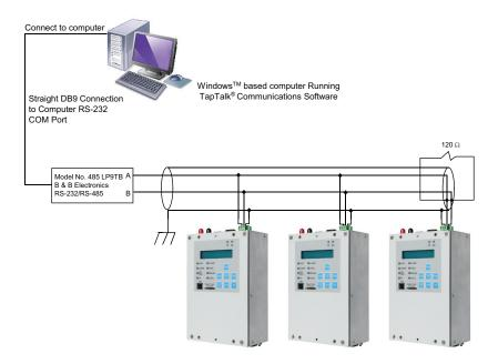
Figure 3. RS-485 Network Connection
