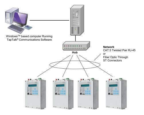
Figure 4. Ethernet Network Connection
