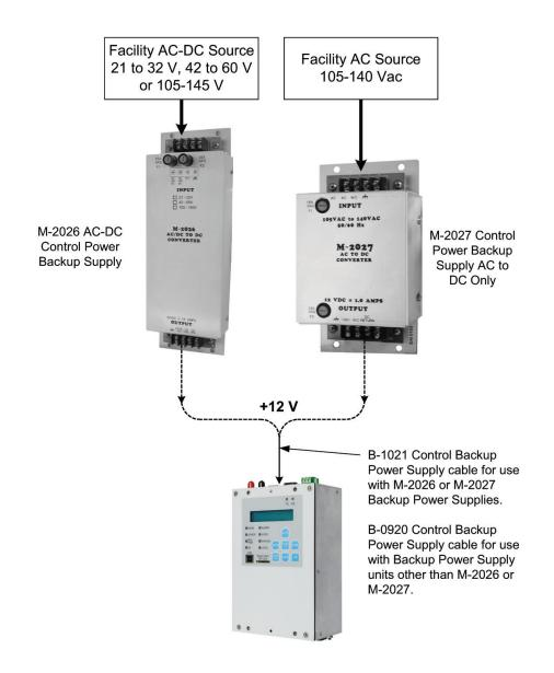
Figure 6. Typical M-2026/M-2027 Control Power Backup Supply Application
