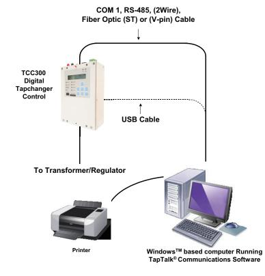
**Communications Using Networking:** The addressing capability of the TCC300 allows networking of multiple ABB Digital Tapchanger Controls. Each tapchanger control can be assigned a Communications Address, Feeder Address or Substation Address ranging from 1 to 65519. Selected commands may be broadcast to all controls on the network. Figures 2, 3 and 4 illustrate typical network configurations. Addresses 1 to 247 can be assigned to MODBUS® and 1 to 65519 for DNP3.0.
