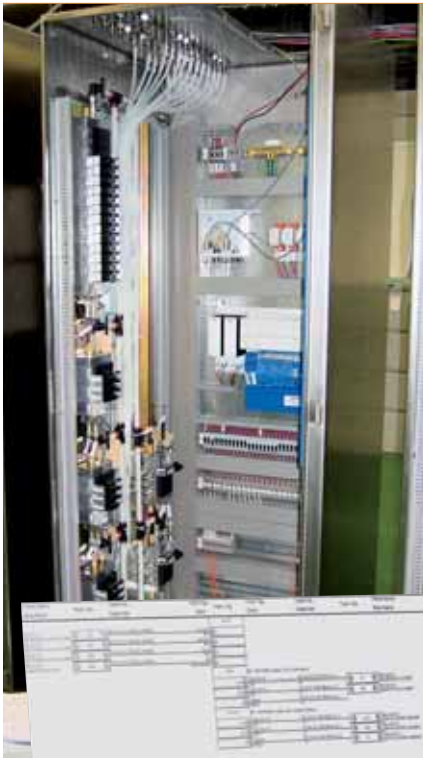
6 Completed cabinet with an example of wiring diagrams automatically generated with PETI
