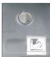
Measuring tap for voltage testing.
