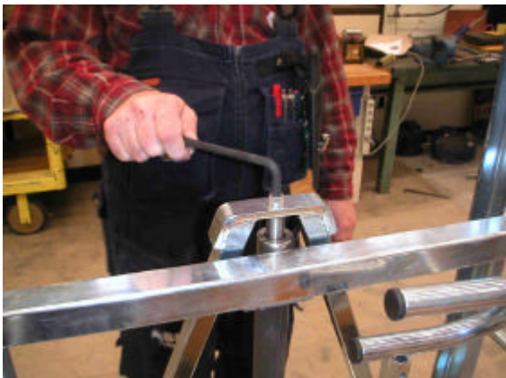
2.9 Mounting the lifting beam on the hydraulic cylinder.
