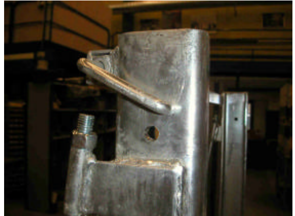
2.6 Pull the locking pin on both sides.
