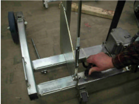
2.5 Use the handle to fasten the wheel.
