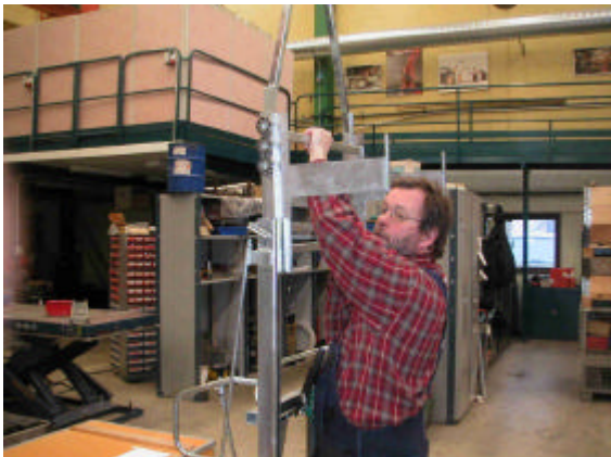
2.7 Mounting the lifting beam.
