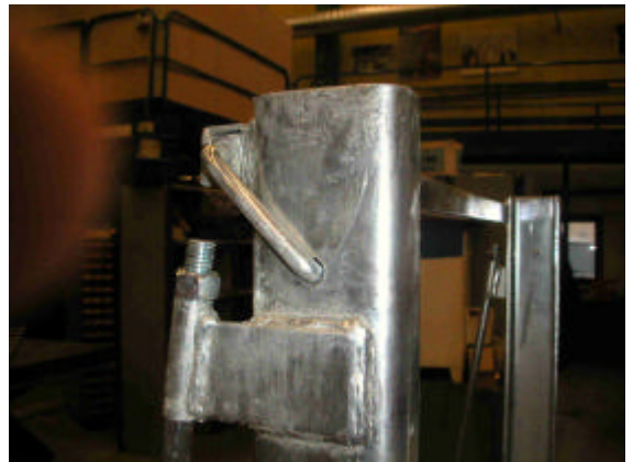
2.8 Lock the lifting beam with the locking pin.
